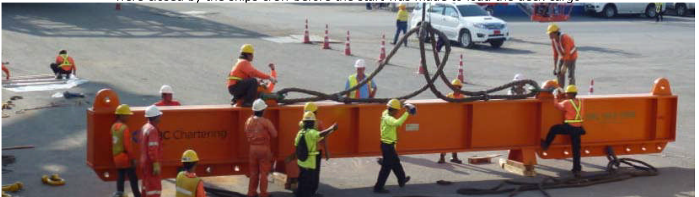
Spreader beams were prepared / rigged up in preparation of the large (volume) lift, the 3800 cub mtr piece with a weight of 218 ton was lifted with 1 crane from the Mammoet transport truck onboard the BBC AQUAMARINE
